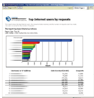
Figure 4: Top Internet Users by Request Shows the top Internet users, the number of individual requests & the total data received. The report is ordered by data received, high to low.
